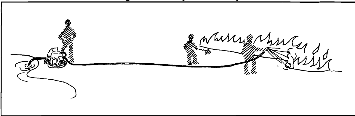
Figure 9—Simple Hose Lay
