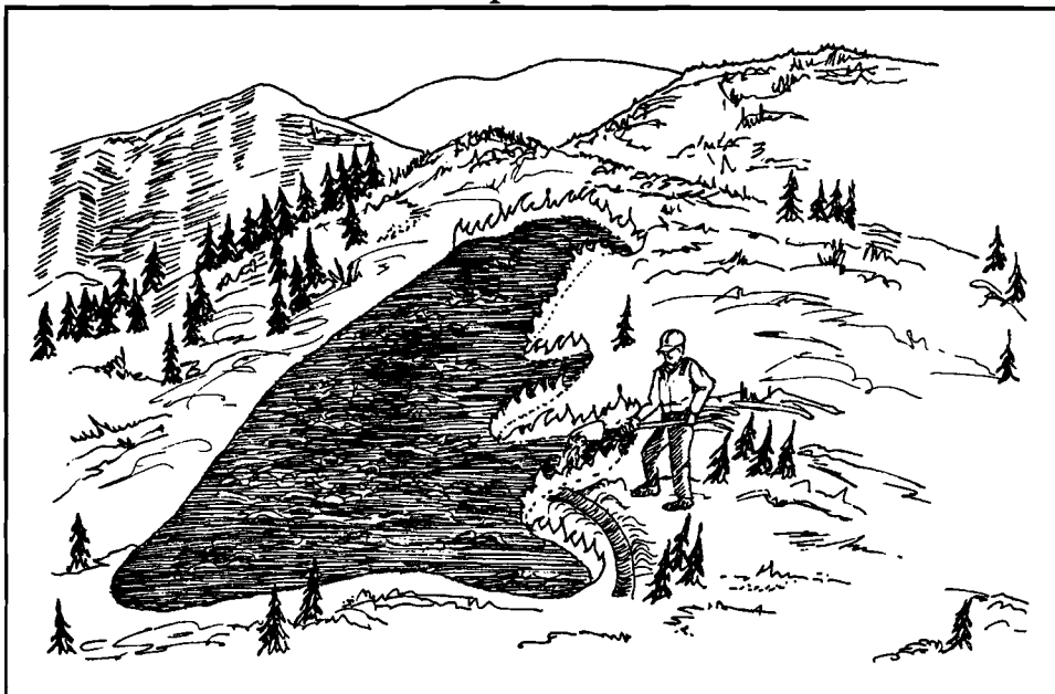
Figure 7—Hotspotting, Using Temporary Lines To Check Fire Spread And Gain Time
