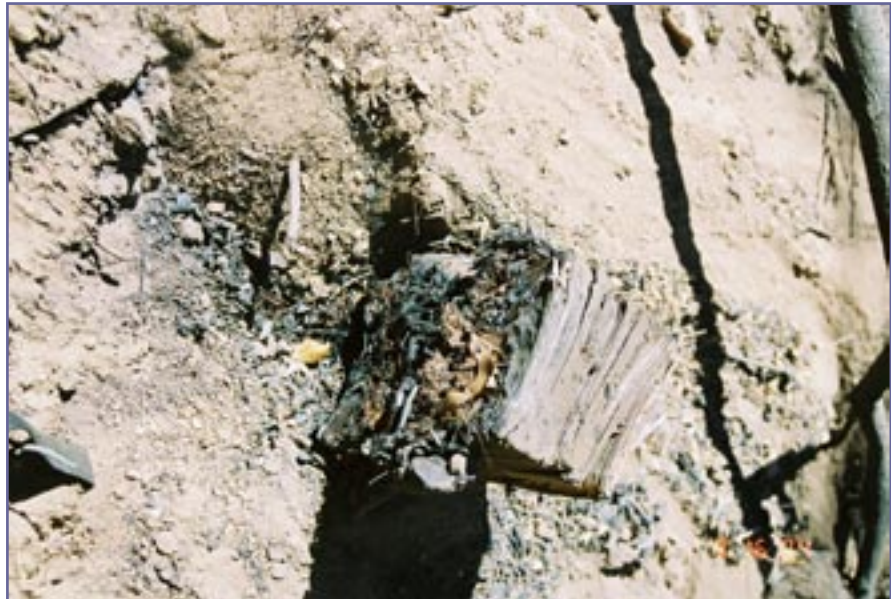
Photo H-22. Photo of fire shelter recovered about 14 feet up-slope from body recovery site. Unburned vegetation attached to and protected by underside of shelter indicates that this area had not burned at the time the shelter reached this location.
